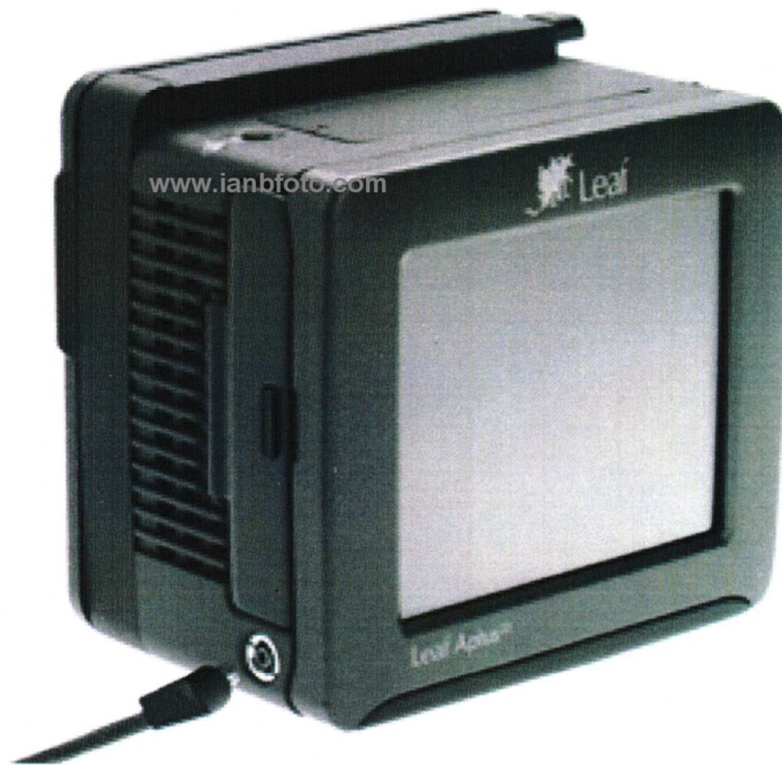
Figure 31: Connecting a Flash Sync Cable to Leaf Aptus
